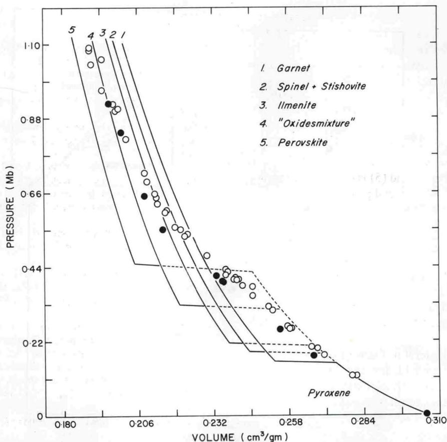
Fig. 4. Analysis of the shock-wave data points displayed in fig. 3 in terms of the possible high-pressure phases of pyroxene. The most probable high-pressure phase of bronzititic pyroxene is "oxidesmixture", as illustrated by the pressure-volume Hugoniot (4) at high pressures.
